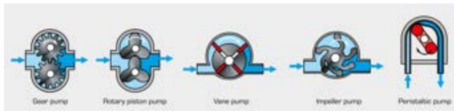
Figure 4: Schematic of some rotary positive displacement pumps
