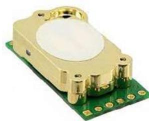
In order to differentiate a healthy patient from a lung cancer patient, a CO<sub>2</sub> supplier was used. When using the normal breath of a person, the T6713 detected a determinate maximum value of CO<sub>2</sub> (ppm). Nevertheless, when the CO<sub>2</sub> supplier was applied, the maximum value of CO<sub>2</sub> (ppm) increased a lot until reaching maximum values unachievable by the human's normal breath.
