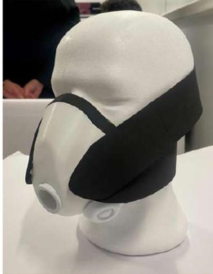
A valve to allow the entrance of external air inside the mask here can be found in both sides of the mask. The hole where there would be the connection between the mask and the big tube also contains a valve that allows the pass of the air to the mass classifier but not the comeback of it.
