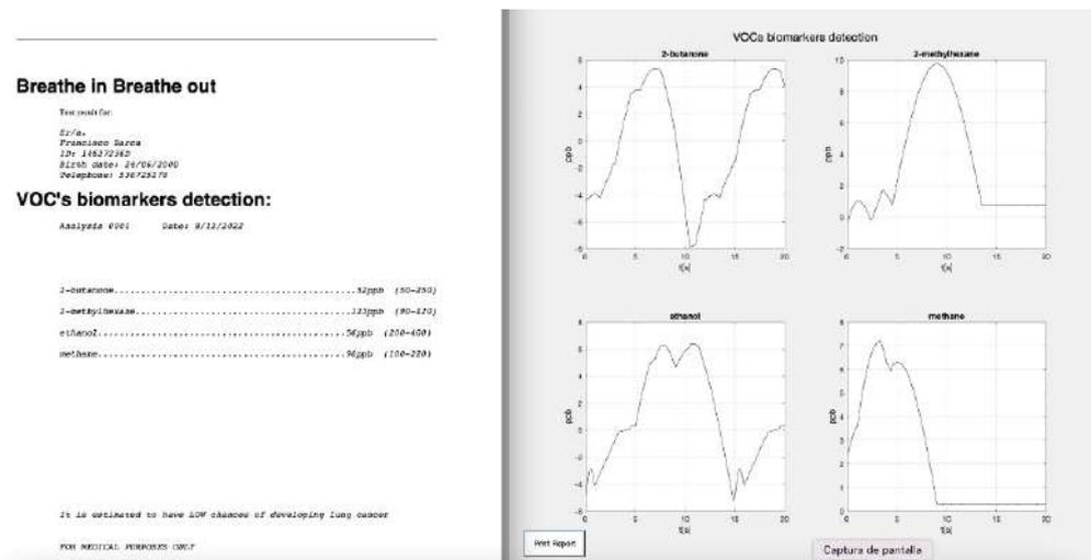
On the right of the image in can be seen the different plots obtained from the values that the chemical sensors send. On the left, the report that will be generated once the test is finished.
