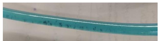
**Fig. 4.** Graphite particles vibrating inside a test tube. Inner diameter is 8.0 mm to allow for easier visualization.
