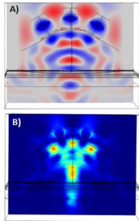
**Fig. 3.** Numerical results of a 3D computer simulation of the ultrasound field generated by the combination of three transducers emitting at 39 kHz in the middle plane. A) Acoustic pressure field (Pa). B) Acoustic power density ( $W/m^2$ ). Higher values are depicted in reddish tones.
