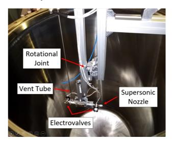
Figure 2: View of the jet propeller prototype, used to measure the generated thrust.
