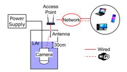
Figure 1 Schematic of the setup demonstrating wireless data transmission.
