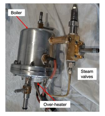
Figure 3: Boiler and over-heater prototype.
